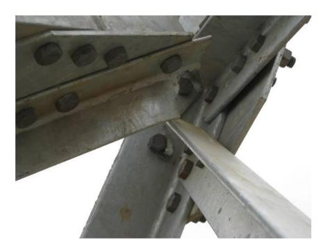
Incorrectly detailed bolt pattern failed during testing of 10 degree angle structure
