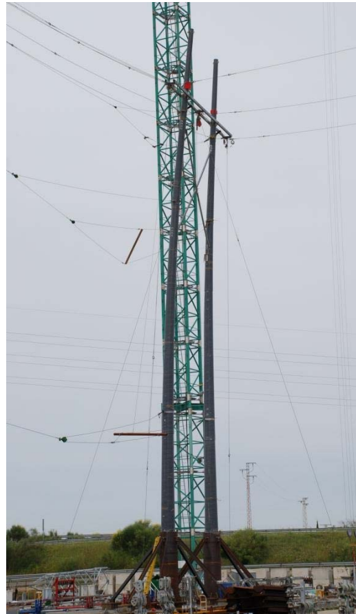
Test #7. Unbalanced Ice-12.7 mm/Bare Ice at -21 Deg. C, No Wind (Tanqent Str.)- Right Phase, L NA+
