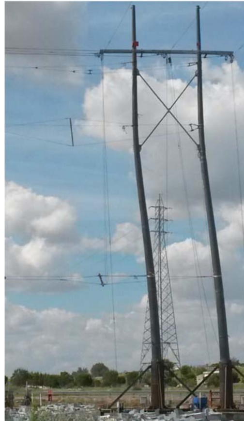
Test #9, High Wind [1320 Pa] With Point Load WR [Tangent Str.], L NA+
