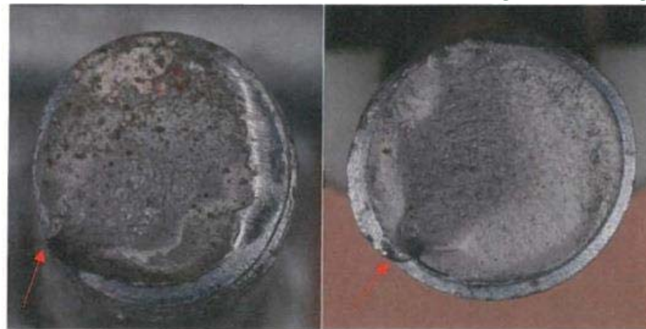
Figure 2. Composite image of the bolt fracture surfaces on: (a) the threaded portion, (b) the un-threaded portion. A shear lip on both surfaces, likely the location of final fracture, is indicated with an arrow.
