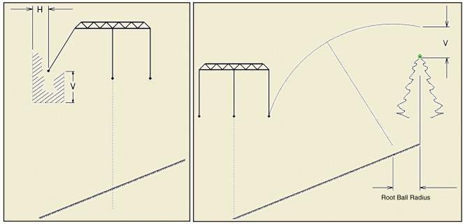
Fig. 3. Vegetation grow-in clearance requirements. Fig. 4. Falling tree clearance requirements.
